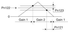
• The settings for the Gain Switching Level in Speed Control (Pn122) and the Gain Switching Hysteresis in Speed Control (Pn123) are enabled absolute values (positive/negative).
