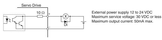
Di: Surge voltage prevention diode (Use a high-speed diode.)
