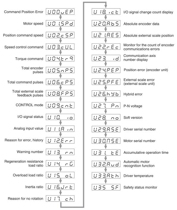
When is pressed, the display position will move in the direction of the arrow.
