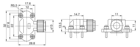
Angle plug model JN8FT04SJ1 (Japan Aviation Electronics) Socket contact model ST-TMH-S-C1B-3500-(A534G) (Japan Aviation Electronics)
