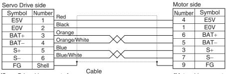
[Servo Drive side connector] Connector model 55100-0670 (Molex Japan)
