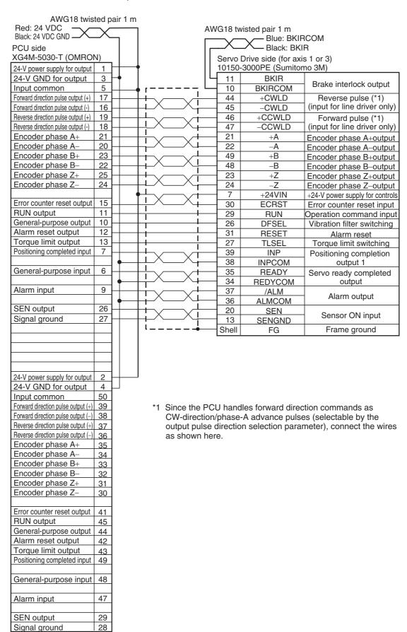
• Cable for open collector output for 1 axis
