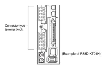
1. Remove the terminal block from the driver before wiring.
