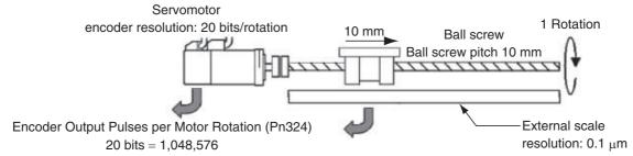
External Scale Output Pulse Per Motor Rotation (Pn325) 10 [mm] / 0.1 [µm/pulse] = 100,000 [pulse]
