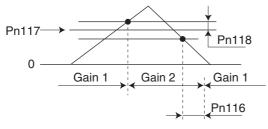
• The settings for the Gain Switching Level in Position Control (Pn117) and the Gain Switching Hysteresis in Position Control (Pn118) are enabled as absolute values (positive/negative).
