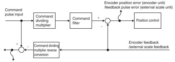
Position command error (command unit) /command feedback pulse error (command unit)
