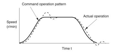
• If the position loop gain is low, positioning completion speed becomes slow.
