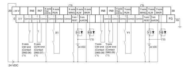
\*1. CW and CCW limit input signals can also be input through Input Units. The signal for the CW/CCW limit inputs in the CJ1M are as follows: CW: A540.08, CCW: A540.09 for pulse output 0 and CW: A541.08, CCW: A541.09 for pulse output 1. Accordingly, the actual inputs can be used as the CW/CCW limit by outputting the flags below in the ladder program.
