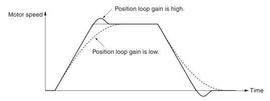
• If the speed loop gain and position loop gain are optimally set, the motor operation for the command will be delayed 2/Kp at acceleration and delayed 3/Kp at deceleration.
