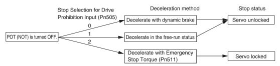
While the Forward Drive Prohibition Input (POT) is OFF, the Servomotor cannot be driven in the forward direction, but it can be driven in the reverse direction. Conversely, while the reverse drive prohibition input (NOT) is OFF, the Servomotor cannot be driven in the reverse direction, but it can be driven in the forward direction.
