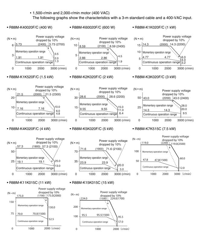
Use the following Servomotors in the ranges shown in the graphs below. Using outside of these ranges may cause the motor to generate heat, which could result in encoder malfunction.
