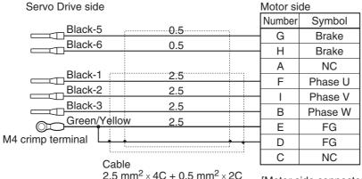
$2.5 \text{ mm}^2 \times 4\text{C} + 0.5 \text{ mm}^2 \times 2\text{C}$
