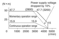
Use the following Servomotors in the ranges shown in the graphs below. Using outside of these ranges may cause the motor to generate heat, which could result in encoder malfunction.
