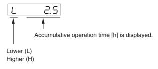
Press to switch between Lower (L) and Higher (H).
