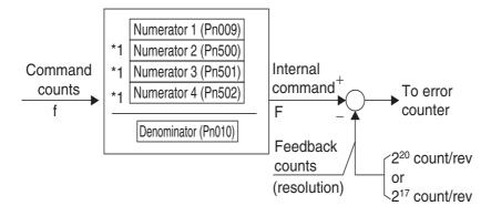
\*1. Numerator 2 to 4 is selected using the electronic gear switching (GESEL1 and GESEL2).
