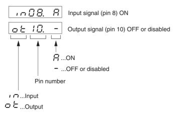
• Displays the status of the control input and output signals connected to CN1.
