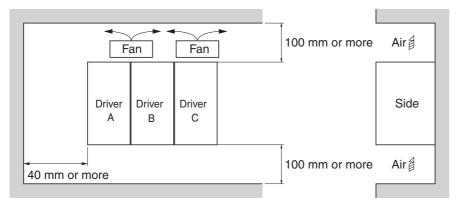
• For side-by-side installation you have to apply next derating for models of 800W or less: Installed in position A, maximum ambient temperature 50°C, installed in position B, maximum ambient temperature 40°C and installed in position C, maximum ambient temperature 45°C.
