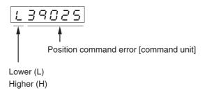
Press to switch between Lower (L) and Higher (H).
