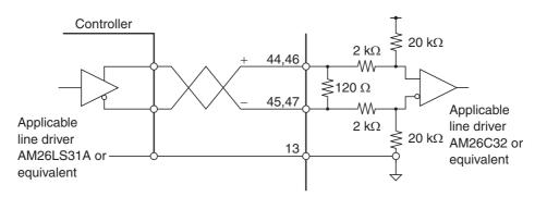
• The shielded twisted-pair cable should not exceed 20 m in length.
