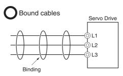
• Separate power supply lines and signal lines when wiring.
