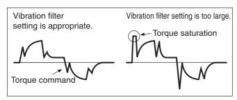
When the Vibration Frequency 1 (Pn214) is set, reduce the setting if torque saturation occurs or increase the setting to increase operation speed. Normally 0 is set.
