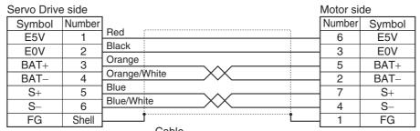
[Servo Drive side connector] Connector model 55100-0670 (Molex Japan) Cable 0.34 mm<sup>2</sup>  $\times$  2C + 0.22 mm<sup>2</sup>  $\times$  2P or AWG22  $\times$  2C + AWG24  $\times$  2P
