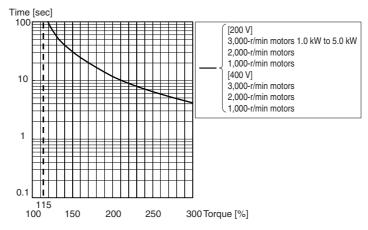
When the torque command = 0, and a constant torque command is continuously applied after 3 or more times the overload time constant has elapsed, the overload time t [s] will be:  $t [s] = -\text{Overload time constant } [s] \times \log_e (1 - \text{Overload level } [\%] / \text{Torque command } [\%])^2$  (The overload time constant [s] depends on the motor. The standard overload level is 115%.)
