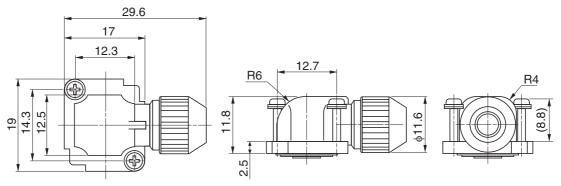
Angle plug model JN4FT02SJ1-R (Japan Aviation Electronics) Socket contact model ST-TMH-S-C1B-3500-(A534G) (Japan Aviation Electronics)
