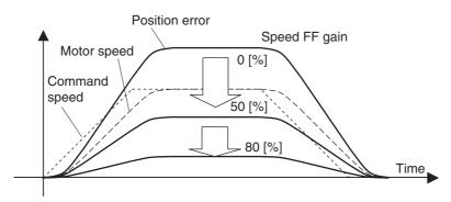
The position error in the range of constant speed becomes smaller as the speed feed-forward gain increases.
