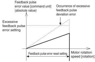
• When using feedback pulse error reset, make sure the feedback pulse error reset setting is set to a proper value. In the case of an extremely small value, it may not function as a protection against error operations caused by erroneous connection of external scale.
