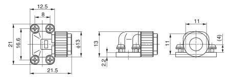
Angle clamp model JN6FR07SM1 (Japan Aviation Electronics) Connector pin model LY10-C1-A1-10000 (Japan Aviation Electronics)
