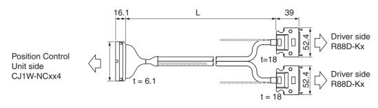
Cable for line-driver output for 1 axis
