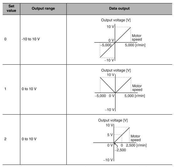
• When monitor type is motor speed and gain of conversion is 500 (1 V = 500 r/min)
