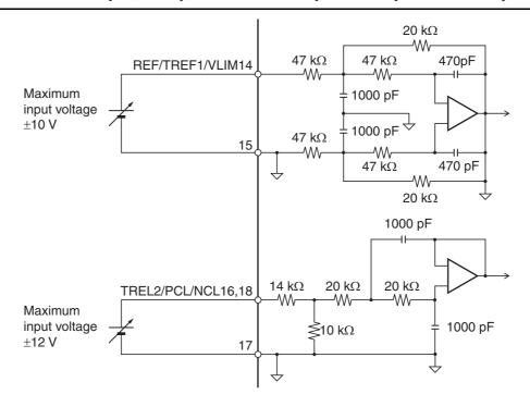
• The maximum allowable input voltage is  $\pm$  10 V for each input. The VR must be 2 k $\Omega$  with B characteristics and 1/2 W minimum. R must be 200  $\Omega$  and 1/2 W minimum.
